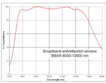
The coatings meet MIL-F-48616: temperature, humidity, mild abrasion and adherence. Manufacturing processes conform to environmental regulations; RoHS (Restriction of Hazardous Substances) EU 2002/95/EC and REACH (Registration, Authorisation and Restriction of Chemicals) EC 1907/2006).
